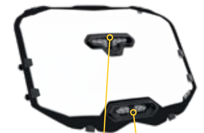
Upper vent channels air into the cabin
